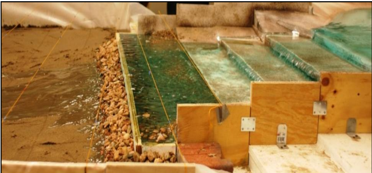
The physical model of the weir allows for test runs of potential stabilization solutions without the expense or manpower involved in physical construction at the actual site.
