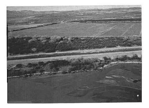
Photo 1 Characteristic features of project area. From bottom to top - river channel, riparian zone, spoil bank levee, conveyance channel, and floodplain vegetation and cultivated land.
