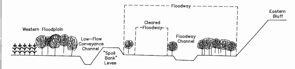
Figure 3. Generalized section of existing floodplain showing location of features. (Not to scale) (After USBR, 1982)
