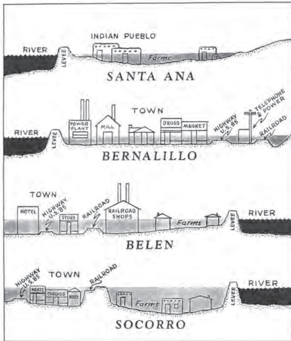
Figure 21. (Opposite) Map and illustrations of middle Rio Grande valley showing national defense installations, transportation routes, important infrastructure features, and communities potentially threatened by Rio Grande flooding. Source: Middle Rio Grande Flood Association (1950).
