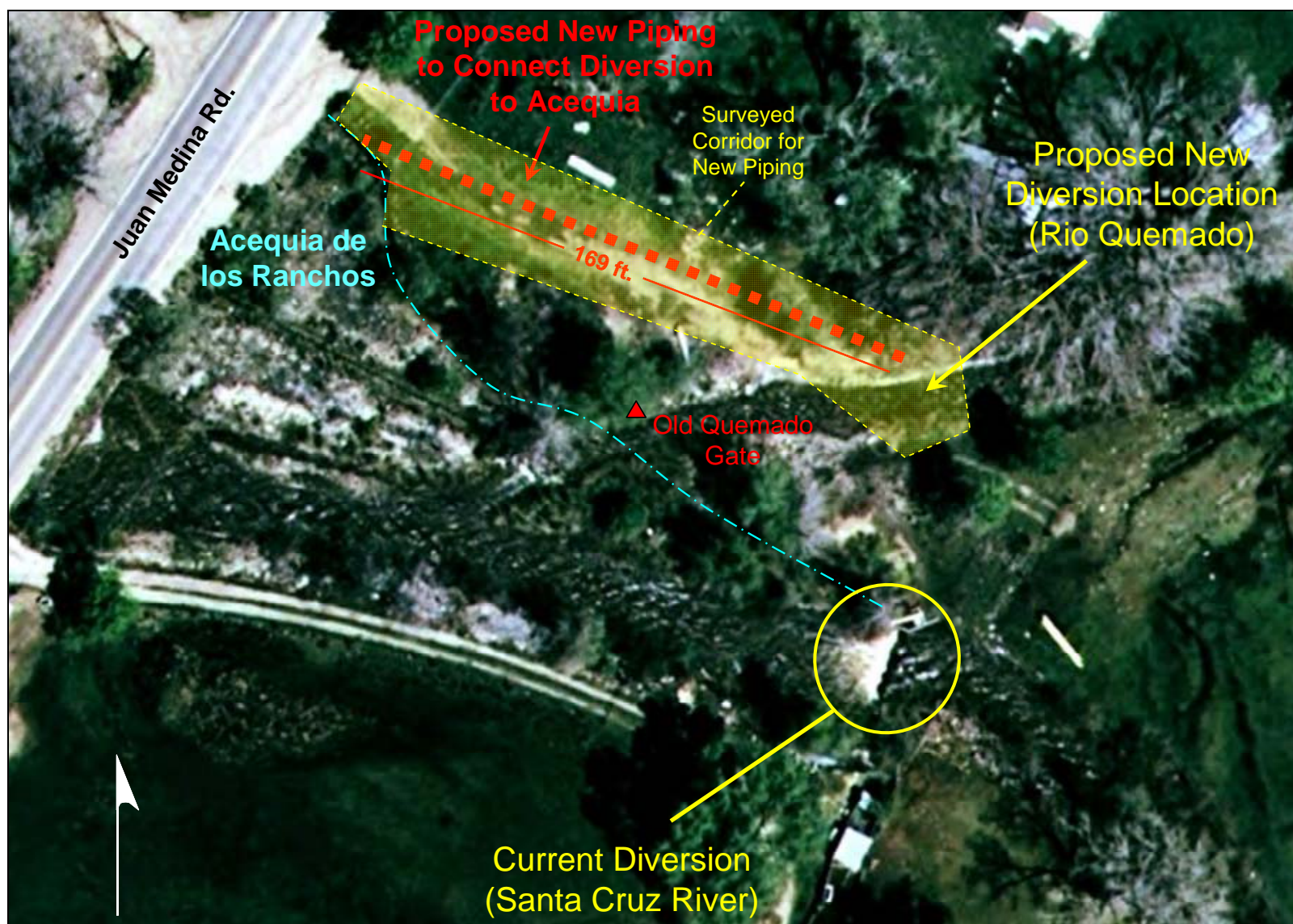
Figure 4.12. Aerial photograph of the Quemado-Santa Cruz confluence vicinity, showing locations of current diversion, proposed new diversion, present acequia alignment, old headgate, and 169 feet of proposed additional piping.
