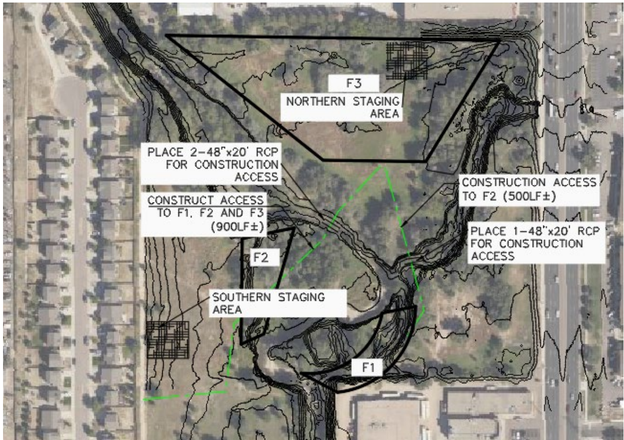
Figure 4: Staging areas and construction route.
