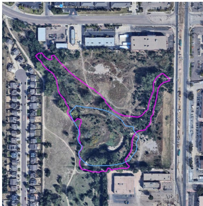
Figure 4 FACStream Assessment Area for Reach 2 (Violet line)(8.65 ac) overlaid with the FACWet Assessment Area for Reach 2 (Blue line)(6.53 ac).
