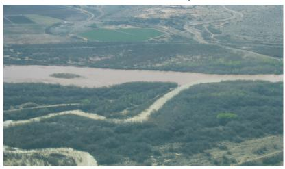
**NARROWS**: River or canal contraction can cause flooding problems upstream as water backs up or downstream if the water bursts the formations causing the contraction.
