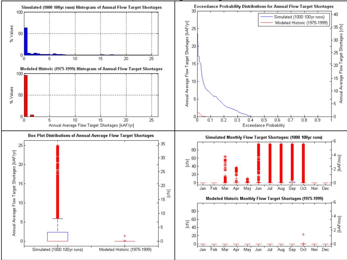
Figure C-23: Stochastic model output for City of Albuquerque San Juan Chama Drinking Water Project shortages (no historic data). These shortages are calculated as the difference between the available allocation as a monthly average, and the amount that is actually diverted. This metric can thus be negative in a given timestep, and ends up counting reservoir evaporation of stored San Juan Chama water as a shortage.
