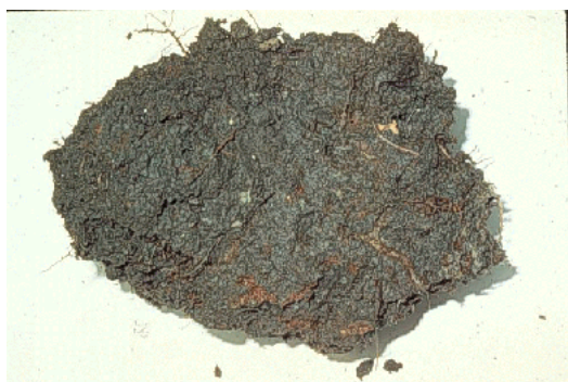
Figure 5. Soil showing matrix (brown) and mottles (reddish-brown)
