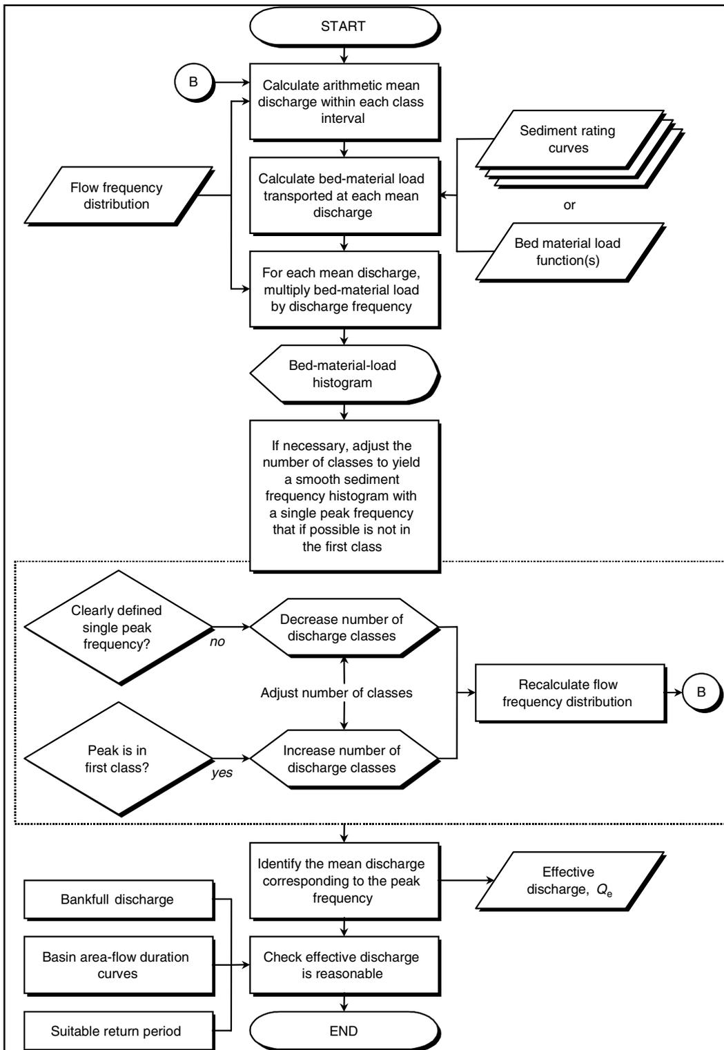
Figure 5. Computational procedure for generating a bed-material-load histogram
