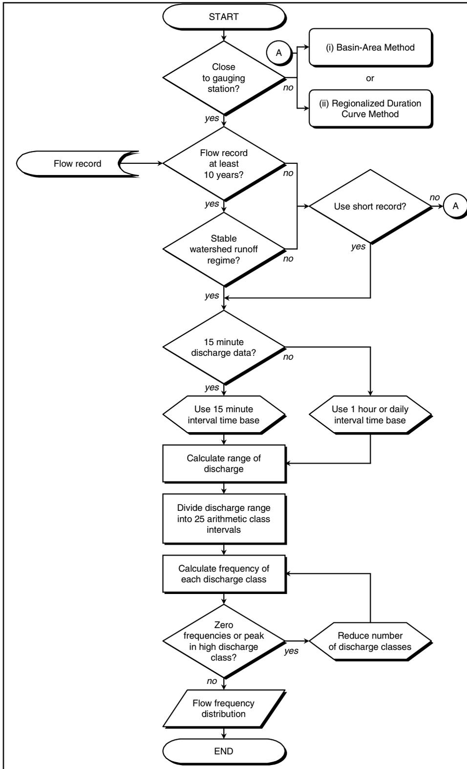
Figure 3. Computational procedure for generating a flow-frequency distribution
