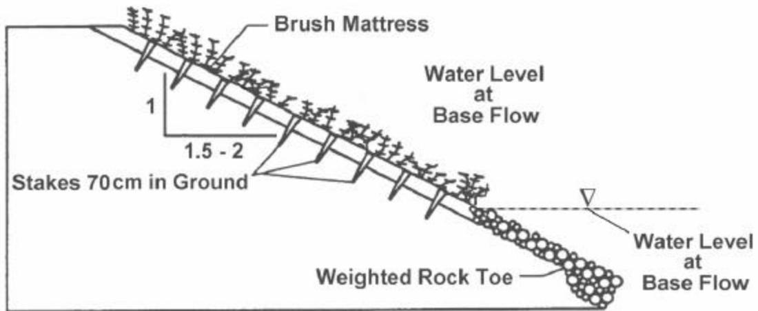
**Figure 2. Profile view of brush mattress with rock toe; note relationship to water level at basal flow and that live brush is not permanently flooded**
